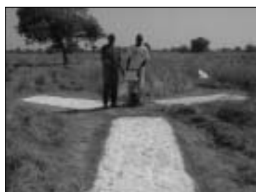
Aerial photo signal ( Y type)
