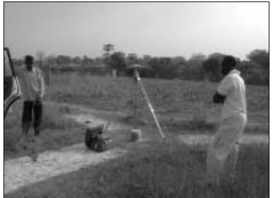
GPS Survey for Photo Control Point
