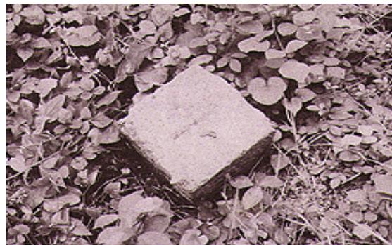
Figure-2 A typical sample of milestone for important points of boundary (triangulation points and benchmarks).
