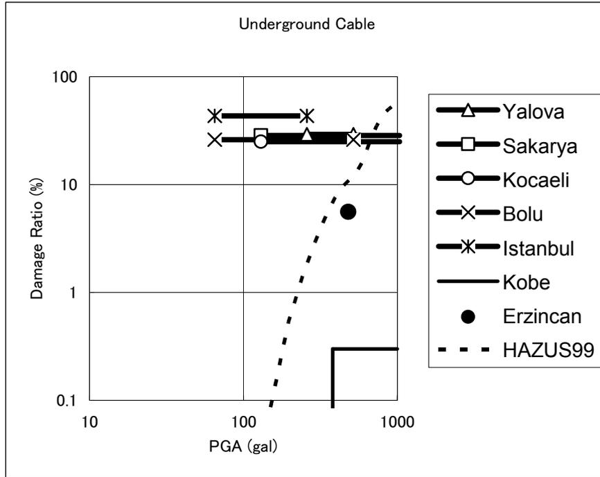
**Figure 9.4.12 Relation between Damage Ratio of Underground Electricity Cable and PGA**
