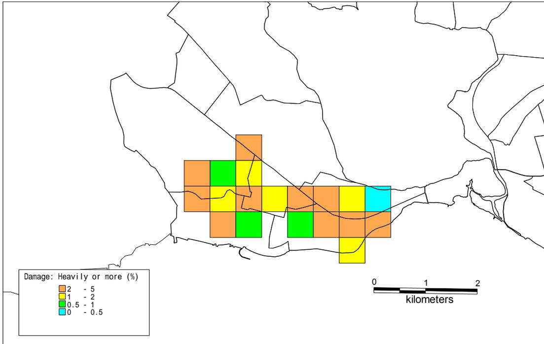
**Figure 6.1.17 Building Damage Ratio by Izmit Earthquake in Avcilar – Heavy Damage or Greater**Source: Avcilar District Office, Compiled by the JICA Study Team
