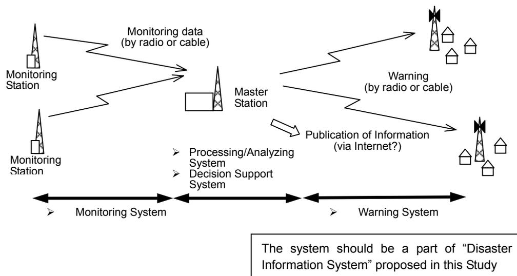
**Figure 5.2.3 Image of Monitoring and Warning System**
