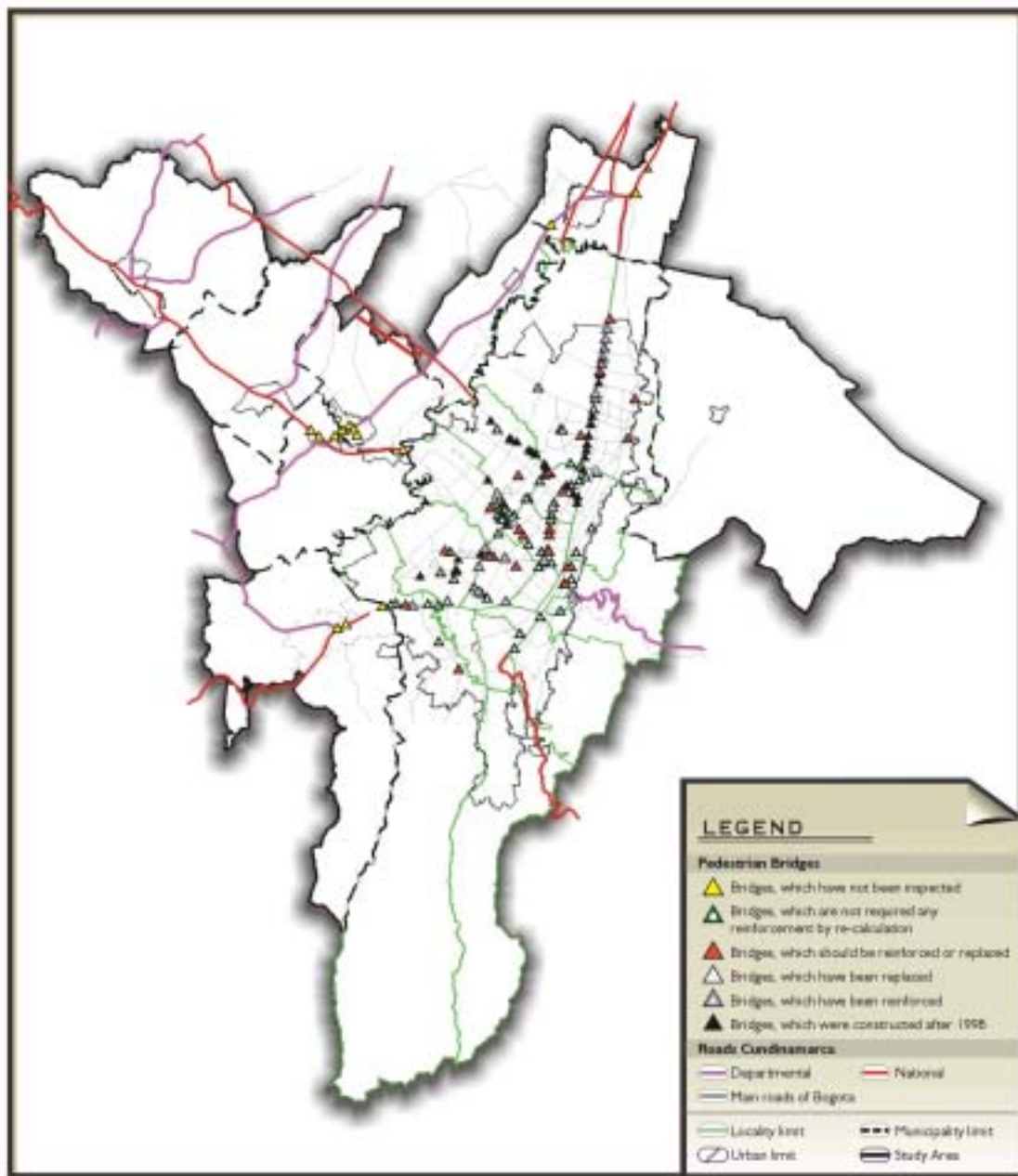
Figure 3.2.7 Pedestrian Bridge Situation according to IDU Investigation 1998
