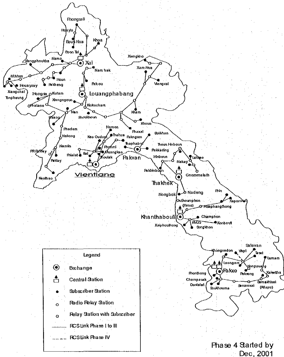
Fig. 12 Overview of Rural Telecom-Networks Phase I to IV
