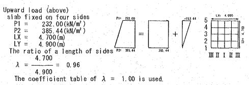
(i)Section force by equivalent uniform load
