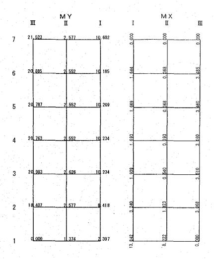
Partition wall (perpendicular to levee normal) Colligation of bending moment
