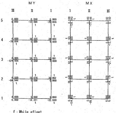
f:While afloat t:Load from a top b:Load from the bottom
