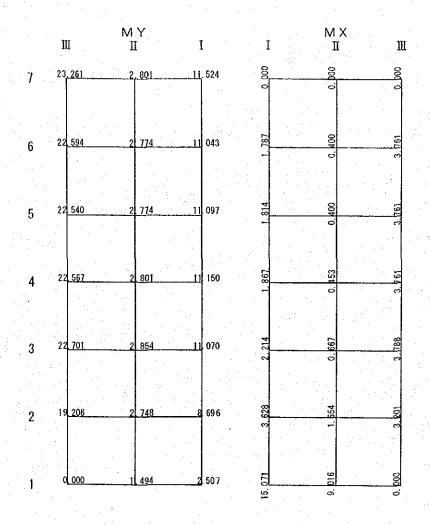
Partition wall (parallel to centerline) Colligation of bending moment
