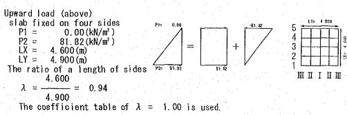
(i)Section force by equivalent uniform load  $P = 81.82(kN/m^2)$
