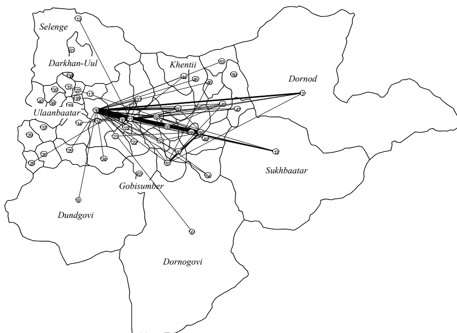
Figure 2-2-3 Desire Line of Existing OD Pairs
