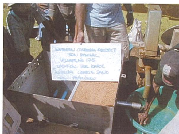
8. Filling coarse sand to D chamber
