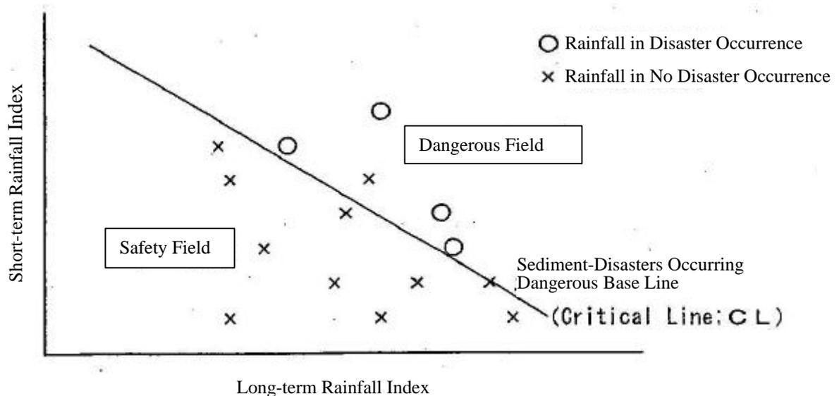
**Figure B.8.2 Concept of Setting Standard Rainfall for Warning/Evacuation of Sediment-Disasters**
