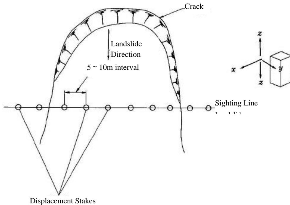
**Figure B.8.4 Layout of Displacement Stakes**
