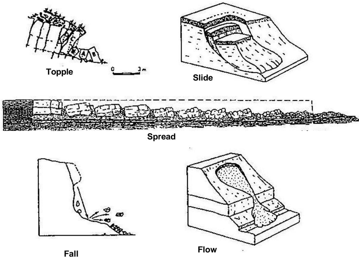
Figure B.6.1 The Classification of a Slope Movement by Vanes(1978)
