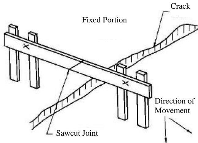
**Figure B.8.3 Typical Observation by the Displacement Board**
