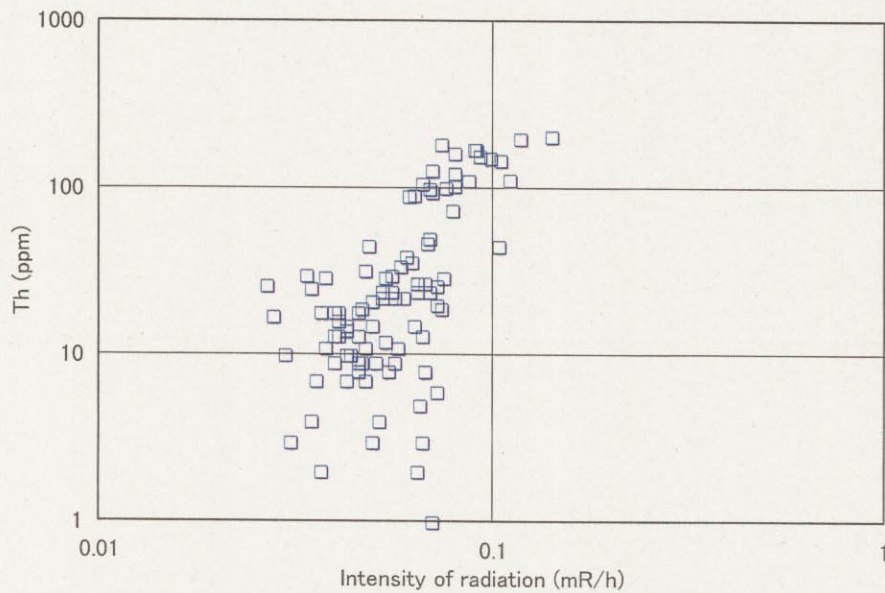
Figure III-4-8 Correlation Diagram between Radioactivity and Th
