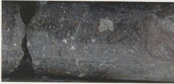
MJVD-19, 24.68m Brecciated limestone
