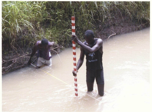
Measurement of river depth (WR11) Width : 4.15m, Max. depth : 0.65m
