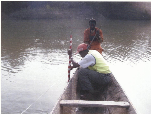
Baoule river Measurement of river depth (WR15) Width : 56.00m, Max. depth : 2.20m
