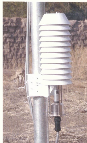
Sensors for temperature and humidity
