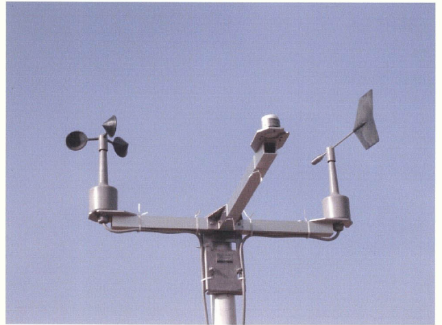
Sensors for wind speed, insolation and wind direction (left to right)
