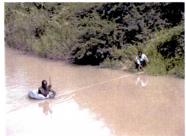
Measurement of flow speed (WR10) Max. depth : 1.25m, Max. flow speed : 0.298m/s
