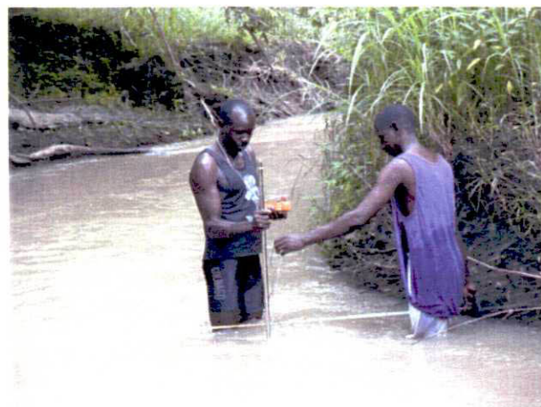
Measurement of flow speed (WR11) Max. depth : 0.65m, Max. flow speed : 0.732m/s
