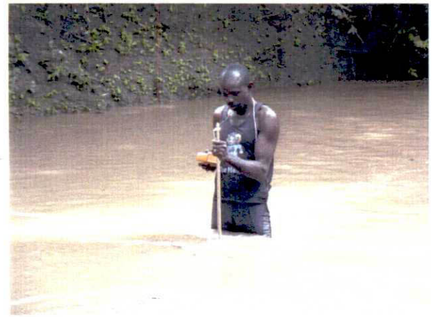
Measurement of flow speed (WR13) Max. depth : 0.80m, Max. flow speed : 0.632m/s
