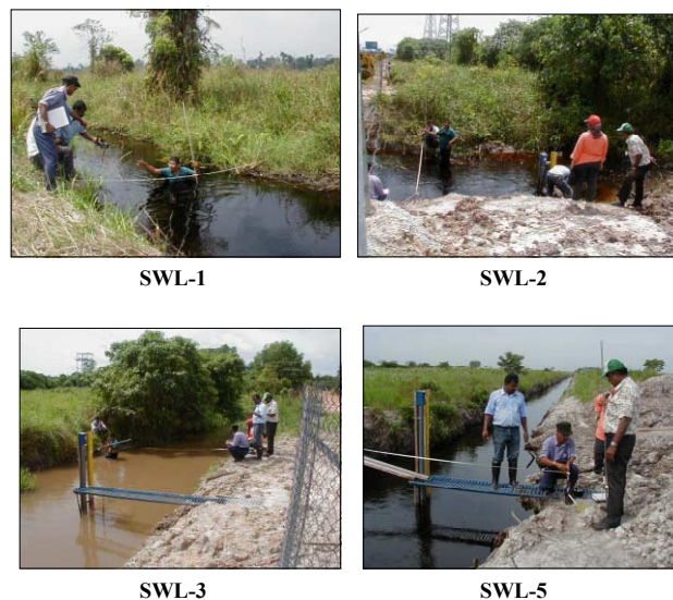
Photograph D.2.1 Measurement of Flow Rate by Cooperation with JPS Gauging Team (Date: 12/12/2000)
