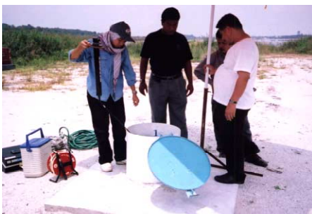
Photo. 3 Taking out data logger and sensor from the well
