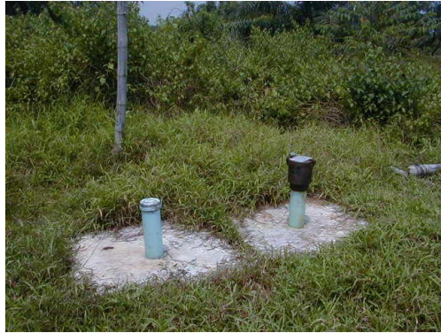
One of Monitoring Wells equipped with Data Logger 29/8/2001
