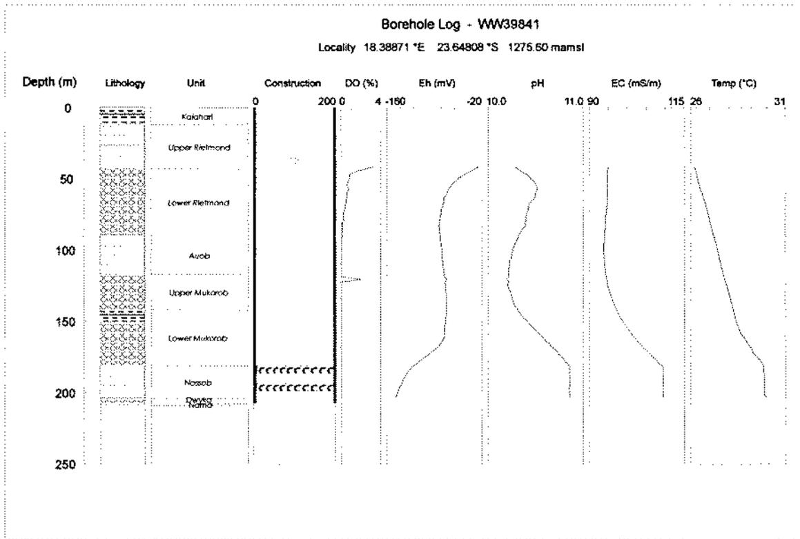
Figure 7.11q Hydrochemical Profiles for Borehole WW39841 (J2N) on Farm Olifantswater West, M102
