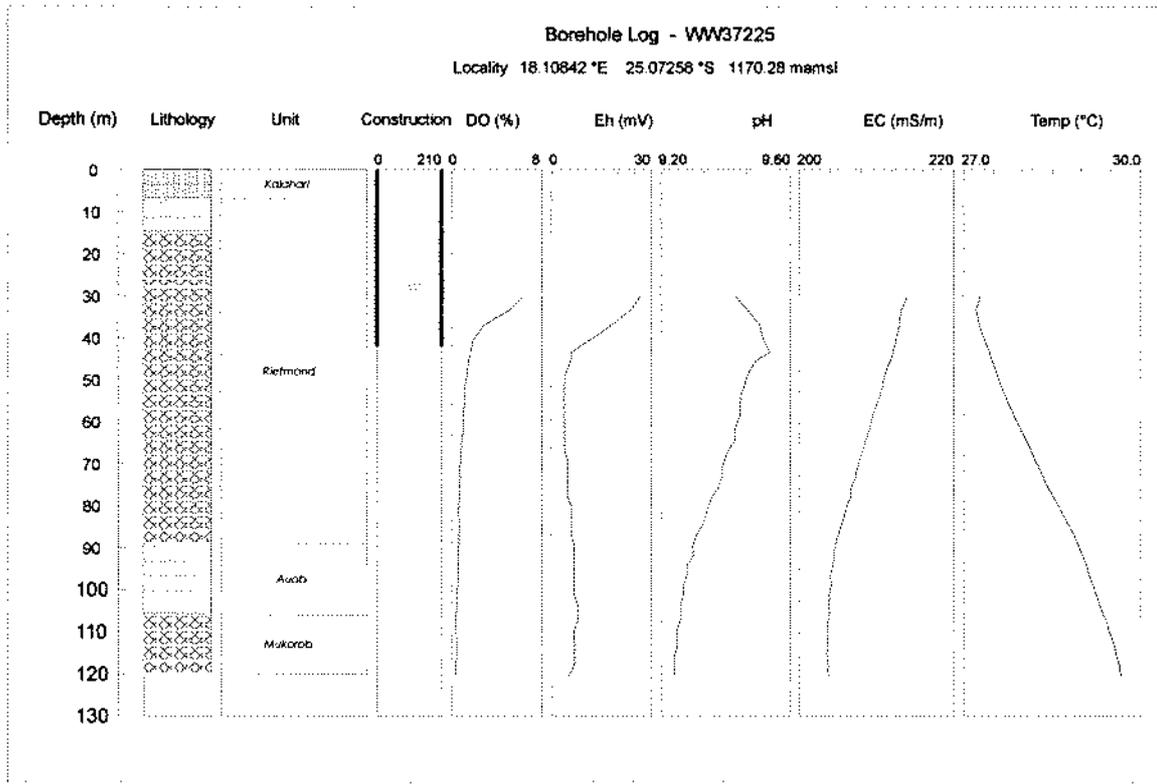
Figure 7.11j Hydrochemical Profiles for Observation Borehole WW37225 (JO-7A) on Farm Glencoe, R78
