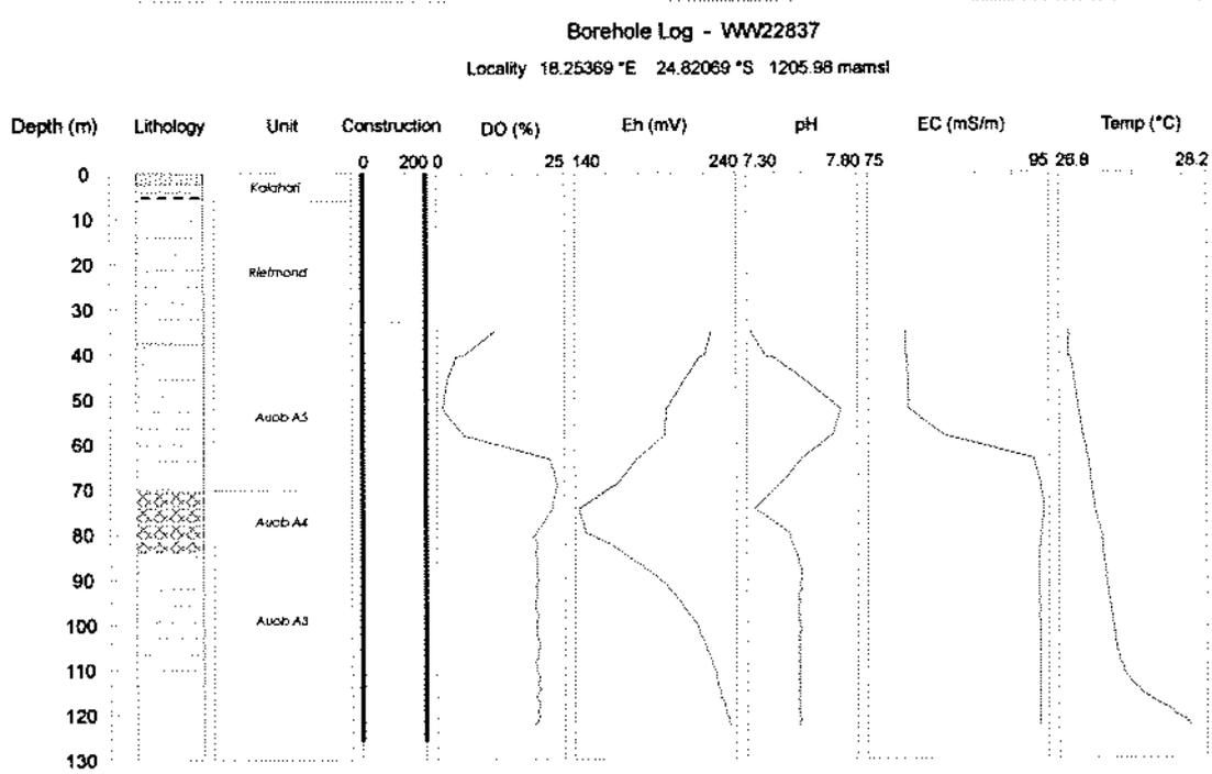
Figure 7.11e Hydrochemical Profiles for Observation Borehole WW22837 (JD-4A) on Farm Tugela, R212.
