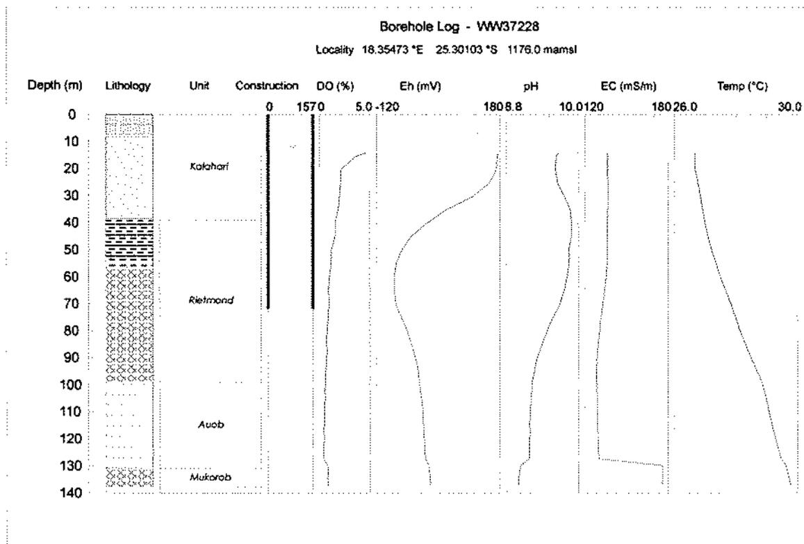
Figure 7.11m Hydrochemical Profiles for Borehole WW37228 on Farm Nootgedacht, R164
