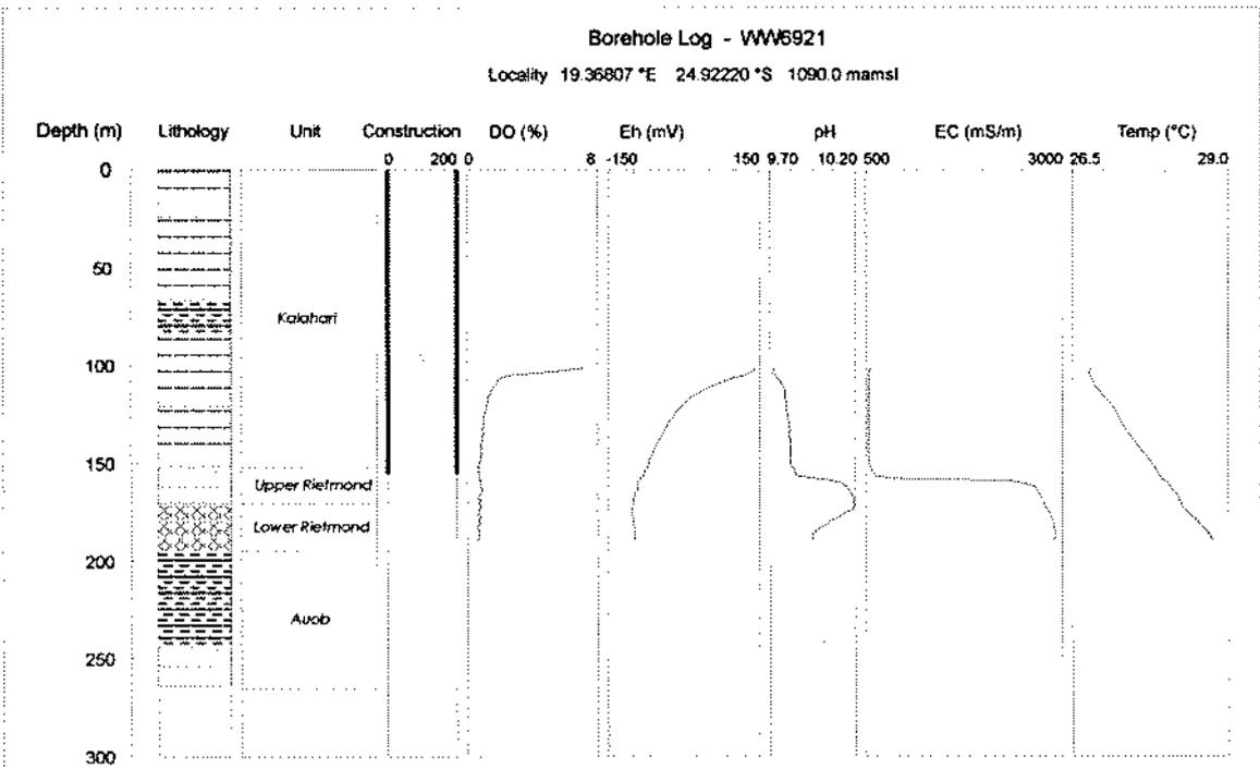
Figure 7.11s Hydrochemical Profiles for Borehole WW6921 on Farm Ou Dempster, R356.
