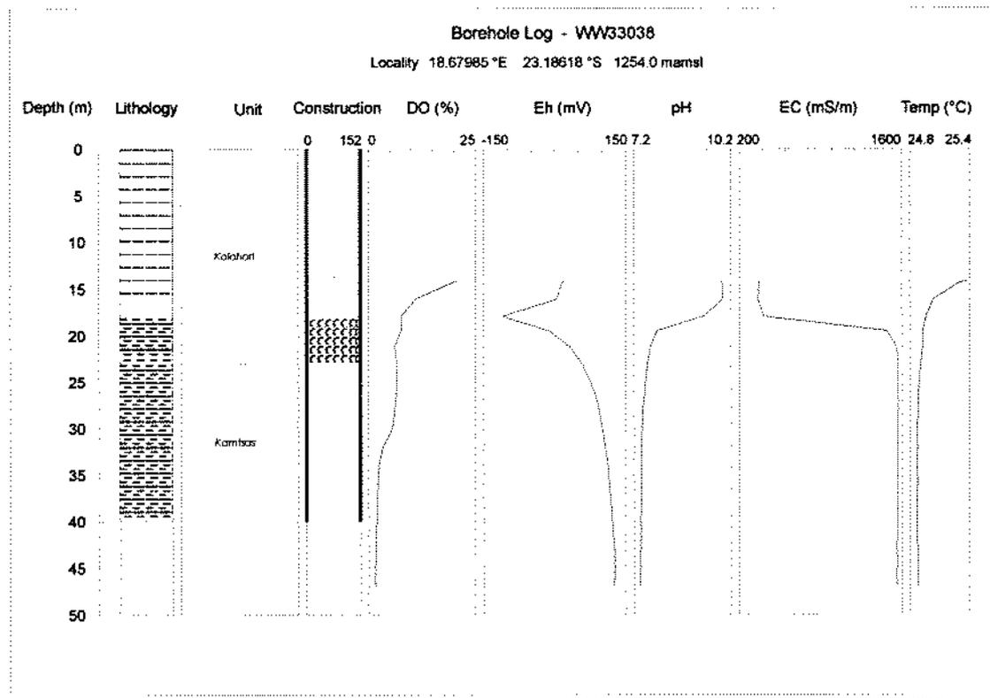
Figure 7.11g Hydrochemical Profiles for Unused Borehole WW33038 on Farm Donnersberg, L29
