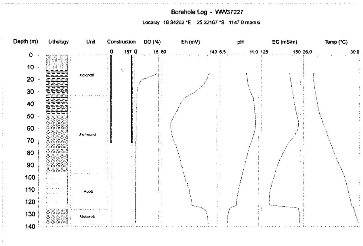
Figure 7.11i Hydrochemical Profiles for Borehole WW37227 on Farm Nootgedacht, R164
