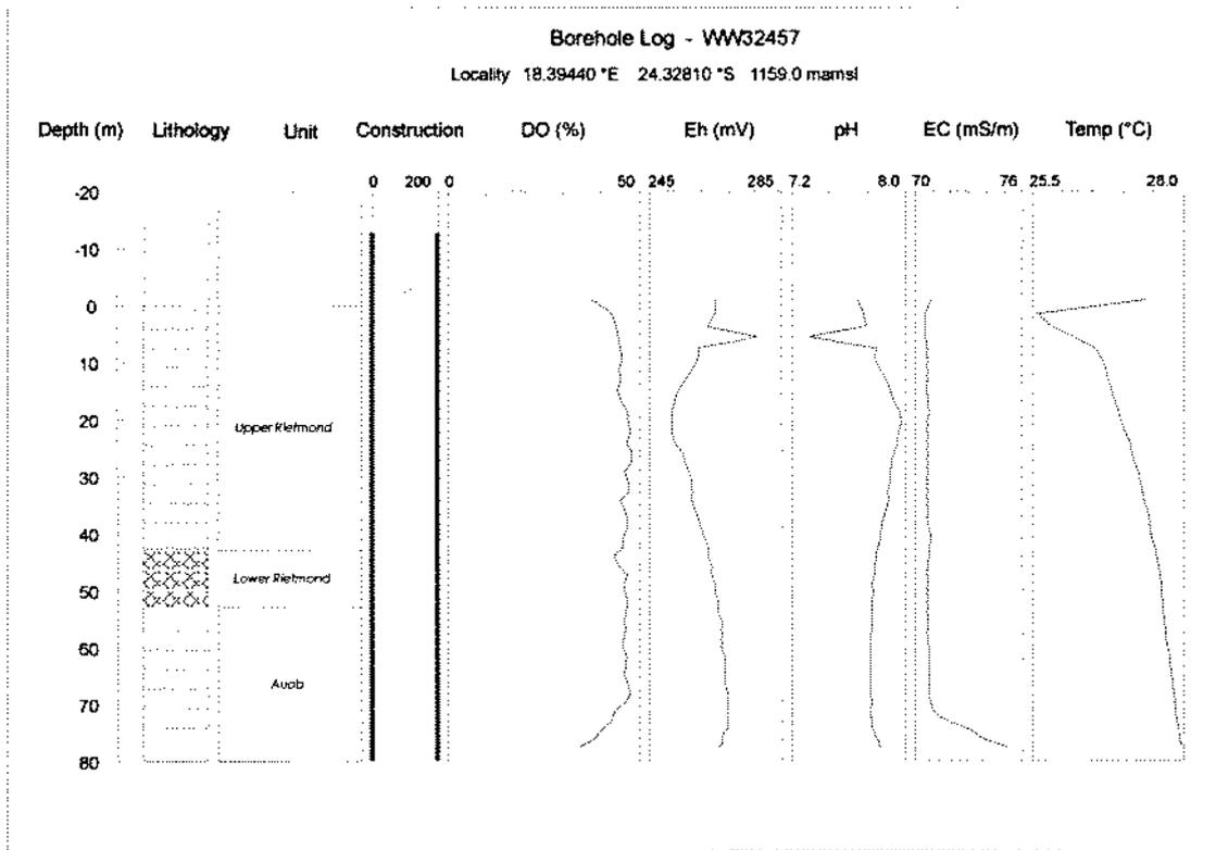
Figure 7.11f Hydrochemical Profiles for DWA Recorder Borehole WW32457 on Farm Spes Bona, R132
