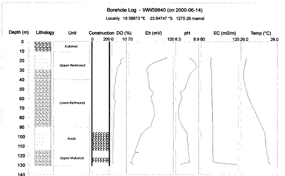
Figure 7.11o Hydrochemical Profiles for Borehole WW39840 (J2A) on Farm Olifantswater West, M102.
