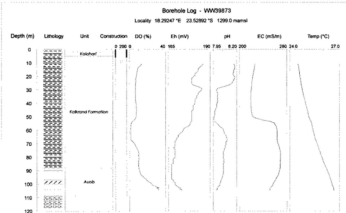
Figure 7.11r Hydrochemical Profiles for Observation Borehole WW39873 (JO-2A) on Farm Gumuchab Ost, M94.
