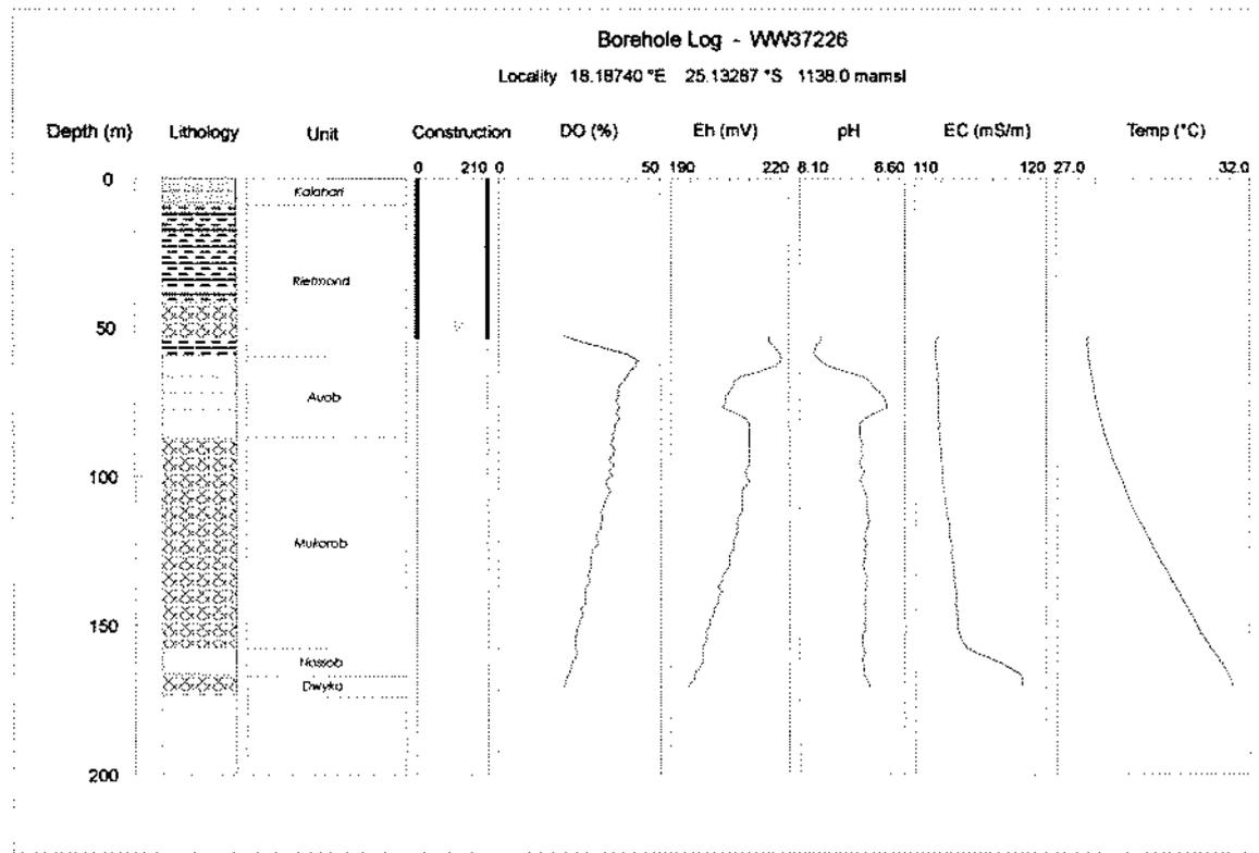
Figure 7.11k Hydrochemical Profiles for Borehole WW37226 on Farm Goamus, R70
