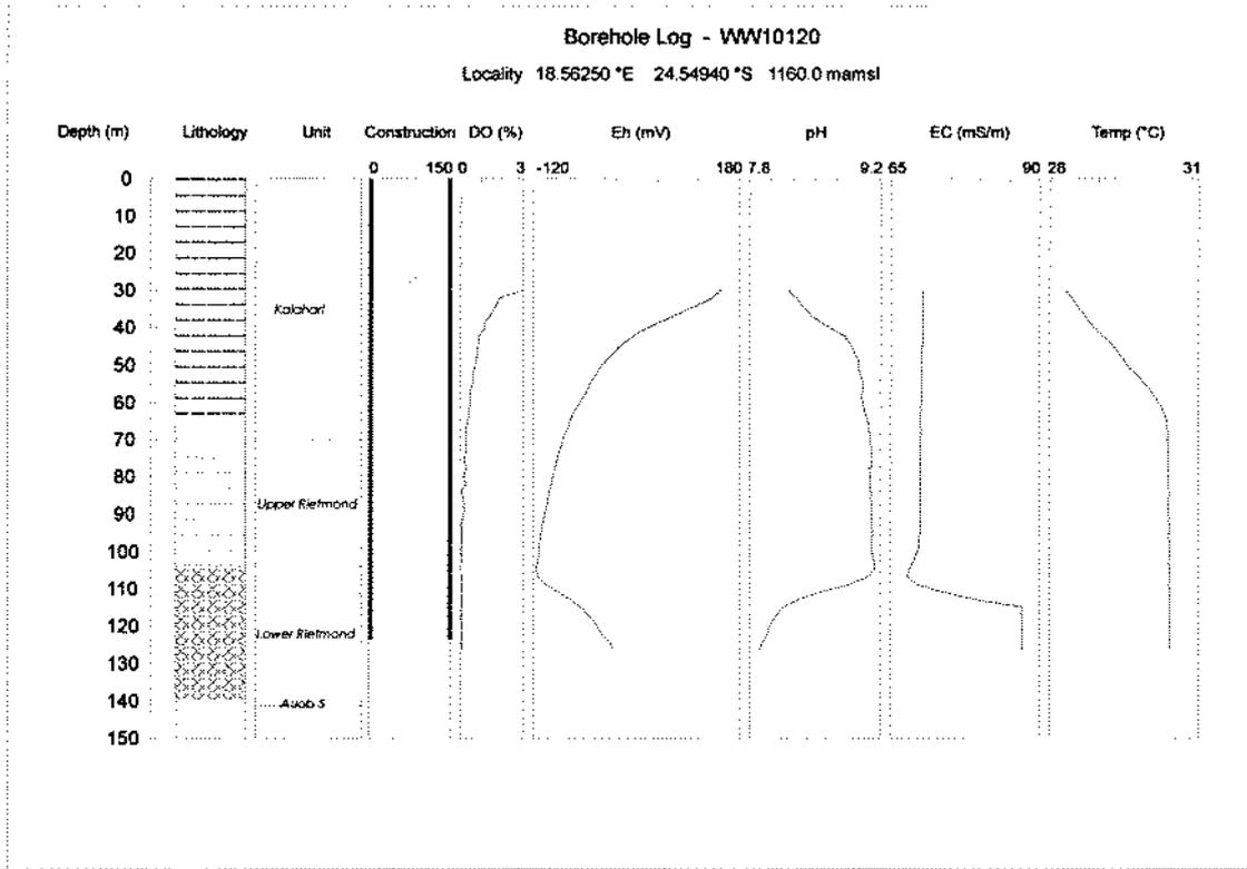
Figure 7.11b Hydrochemical Profiles for DWA Recorder Borehole WW10120 on Farm Boomplass, R386
