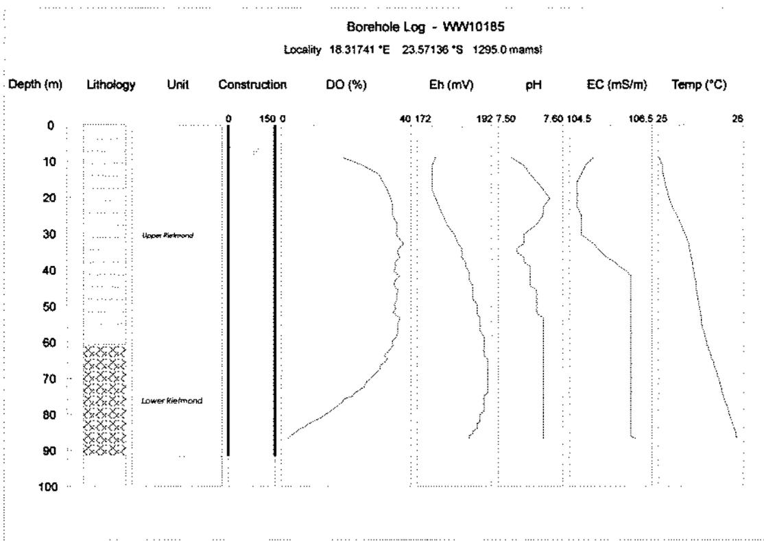
Figure 7.11c Hydrochemical Profiles for Borehole WW10185 at the Roads Camp on Farm Neu Loore, M97
