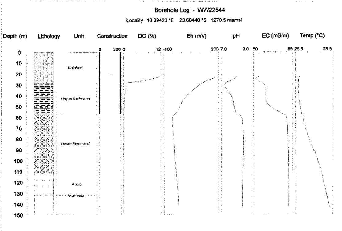
Figure 7.11d Hydrochemical Profiles for DWA Recorder Borehole WW22544 on Farm Olifantswater West, M102.
