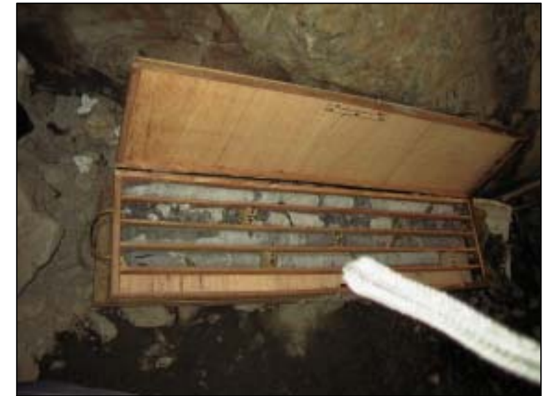
Morro de Arica Dam Site-3: Boring core
