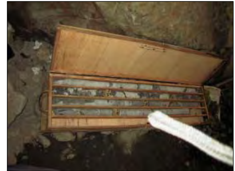
Morro de Arica Dam Site-3: Boring core
