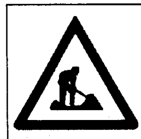
A,16: Road Works Ahead DPWH Code: W6-1
