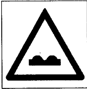
A,7 a : Uneven Road DPWH Code: W5-2
