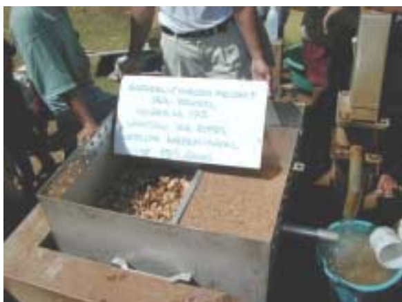
9. Filling medium gravel into C chamber
