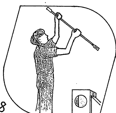
15 SEPARATE FOOT VALVE FROM THE VALVE ROBBIN
