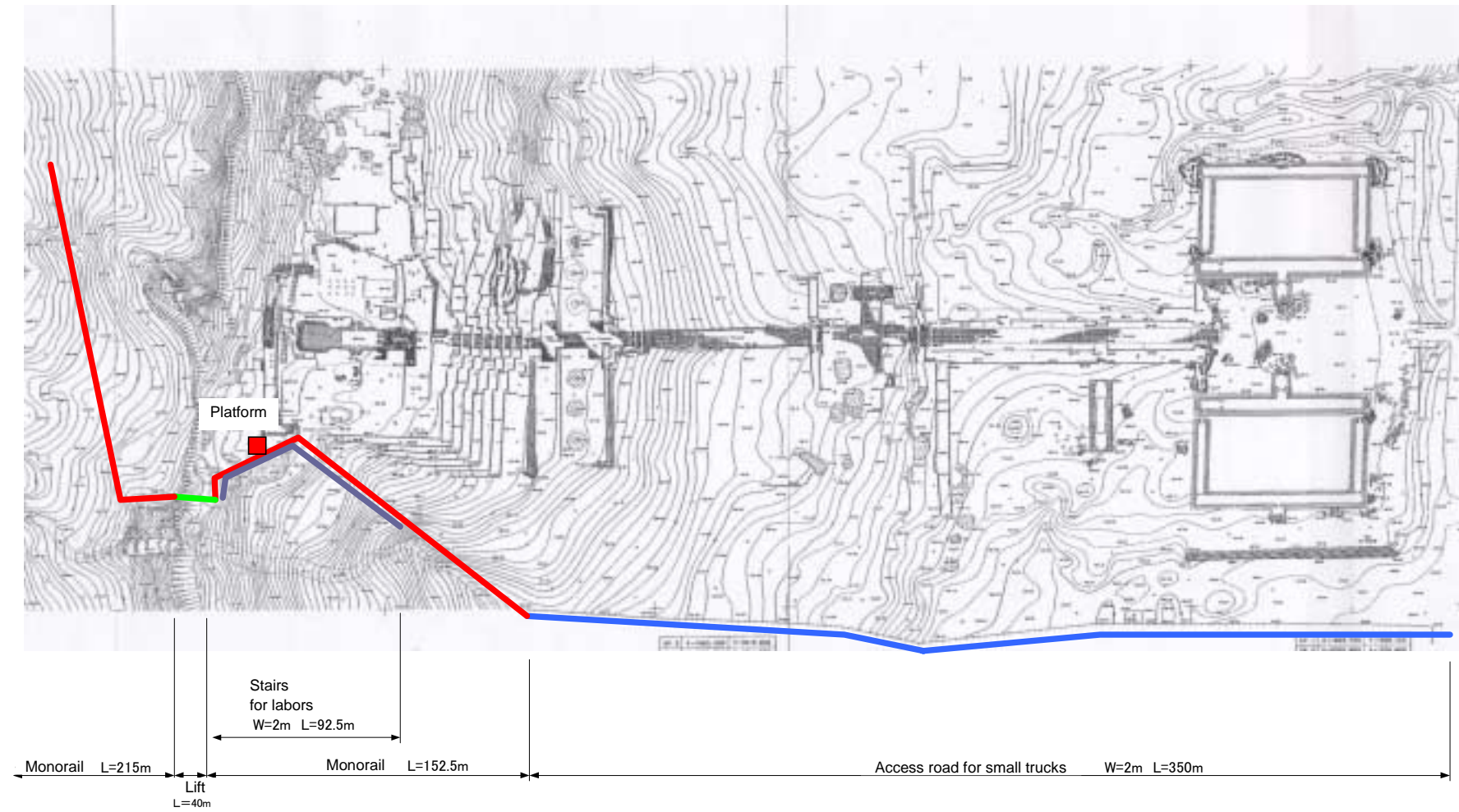
Figure 2-9 Plan of Temporary Transporting Route
