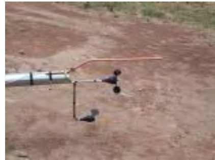
Anemometer, Wind Vane and Lighting Rod
