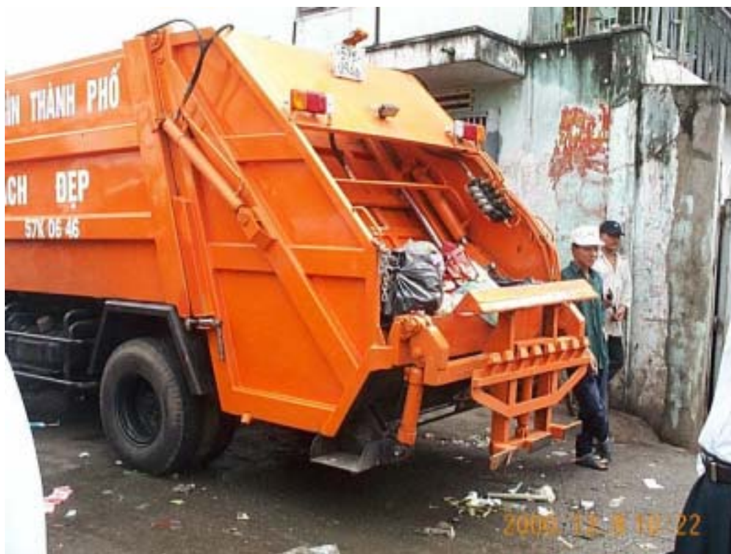
Photo 5: A Recommended Compactor equipped with mechanical lifting device (Used in Hochiminh City)
