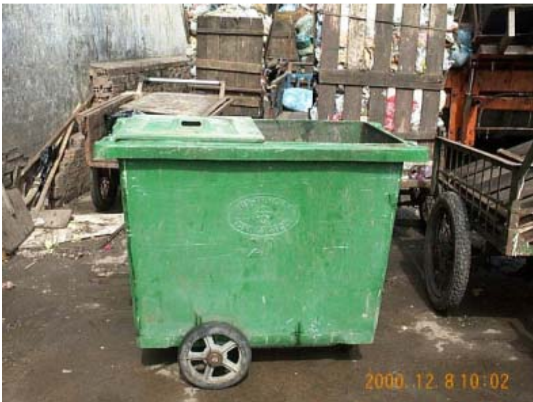
Photo 2: Recommended 660-Liter Bin (This can be used as either fixed location bin or handcart.)
