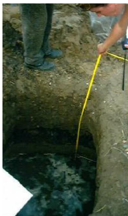
Photo Trial pitting, encountered with Cables and Groundwater
