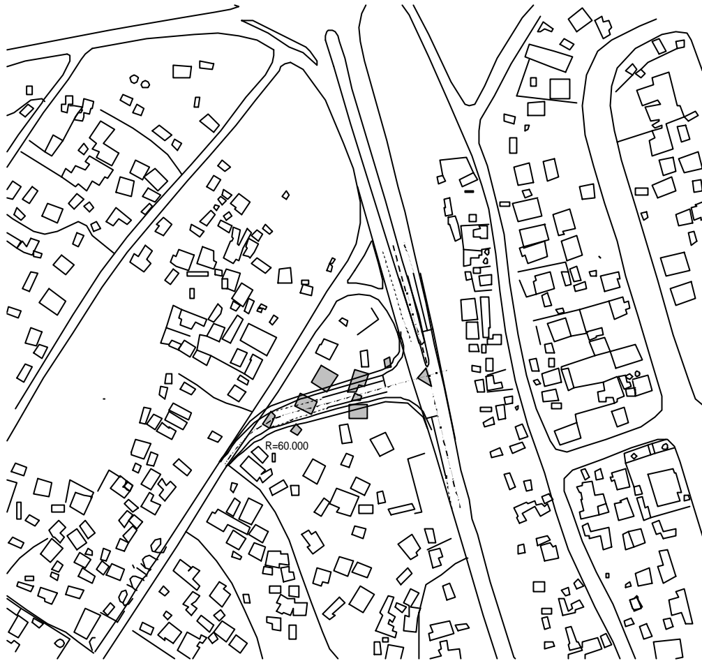
Figure 18.5.3 Draft Plan of T-shaped Intersection at North end of Av. Vladimir Lenine
