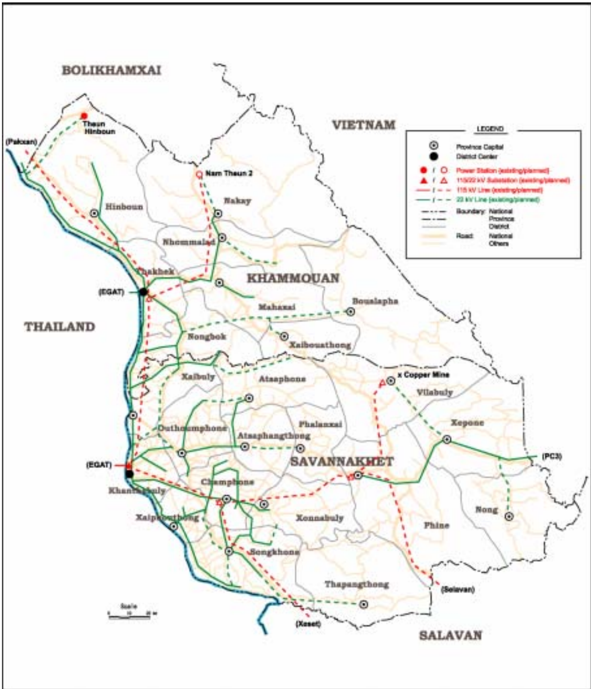
Figure VI3-6 Existing and Planned Distribution System in Study Area
