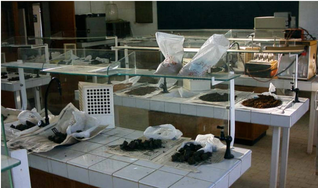
Photo No.61 Soil Preparation (Air Dry)
