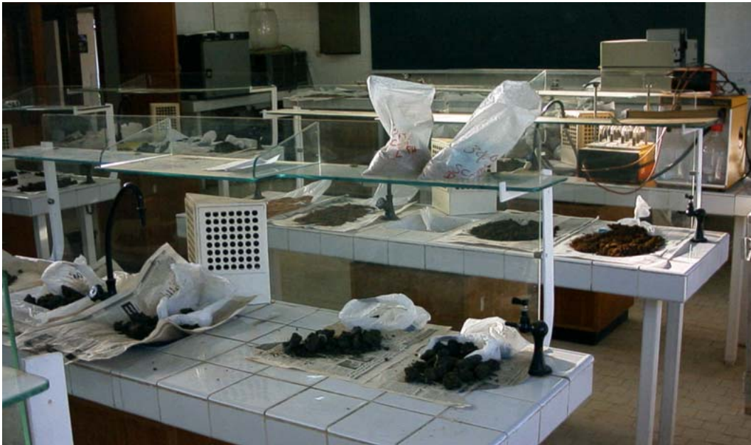
Photo No.61 Soil Preparation (Air Dry)
