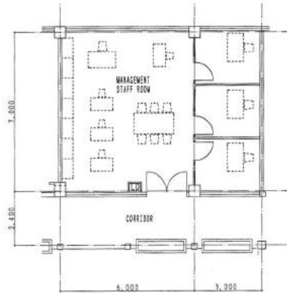
Figure 2-3-6 Management Staff Room
