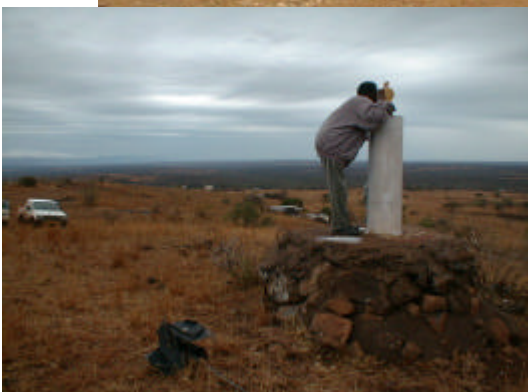
Measurement of elements of eccentricity at a triangulation
