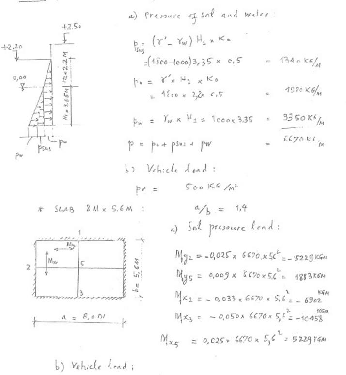
$M_{y2} = -0.051 \times 500 \times 5.6^{2} = -800 \times GM$   $M_{y5} = 0.018 \times 500 \times 5.6^{2} = 282 \times GM$   $M_{x41} = -0.083 \times 500 \times 5.6^{2} = -1301 \times GM$   $M_{x3} = -0.083 \times 500 \times 5.6^{2} = -1301 \times GM$   $M_{x5} = 0.044 \times 500 \times 5.6^{2} = -0.043 \times GM$
