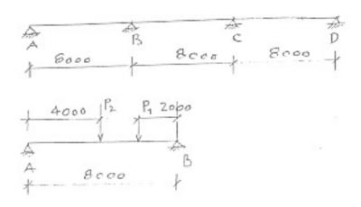
\* SPAN BC AND CD:  $M_{\circ} CD = \frac{1750 \times 8^{2}}{8} + \frac{1250 \times 3.5}{2} \left[ \frac{8^{2}}{4} - \frac{35^{2}}{3} \right] \times 2$   $= \frac{66.135 \, \text{KGM}}{66.000} = \frac{M_{\circ}}{8} \text{C}$
