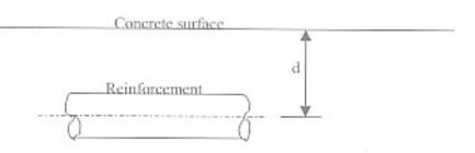
Underside of bottom slab d = 120 mm (with pile structure)
