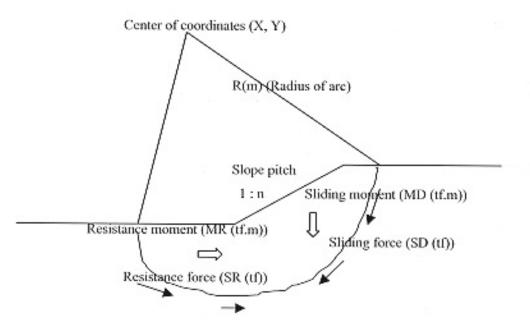
The calculation is done to meet a minimum safety factor in condition of assumed coordinates (X, Y) and radius of are (m). Also each soil condition is considered.
