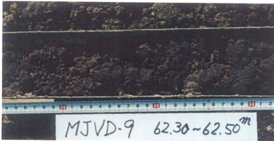
P.3 MJVD-9 62.30~62.50m strongly weathered black ore (TRE 2 O 3 :3.36%, CaF 2 :26.92%, BaSO 4 :13.09%)
