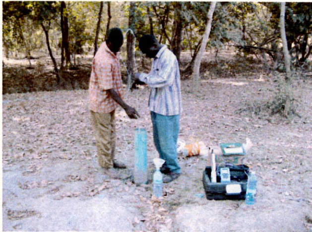
Water sampler is moved down in the hole of MJMB-E3. Inner diameter of PVC casing is 126mm.
