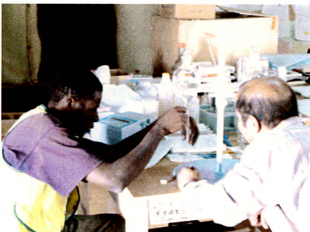
Analysis for water (pre-treatment for Ni) Ejecting liquid reacted in the separating funnel to the container for measurement.
