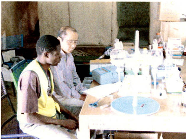
Analysis for water (pre-treatment for Ni) Waiting for reaction time in the separating funnel.
