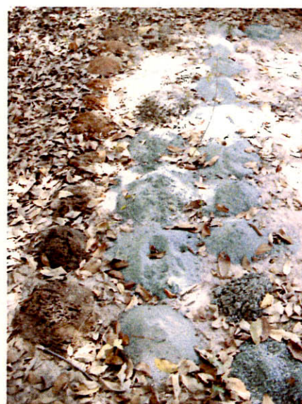
Cuttings of MJMB-E3 (0~31m) Unconsolidated sediments from the top to 15m deep, granodiorite to the bottom
