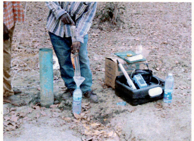
Underground water is collected from the hole of MJMB-E3. Equipment in the right side can measure pH, temperature, conductivity, DO and turbidity.
