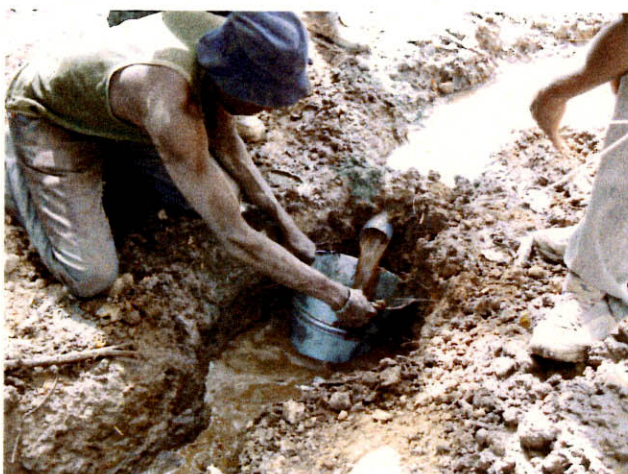
MJMB-E3: Measurement for water amount pumped The amount is about 3 t/h.
