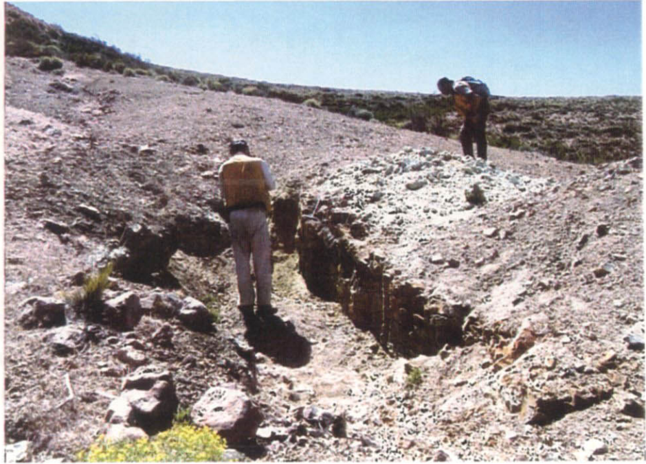
Plate 21 Campana Mahuida district : A short trench with a stock pile of barite ore with malachite
