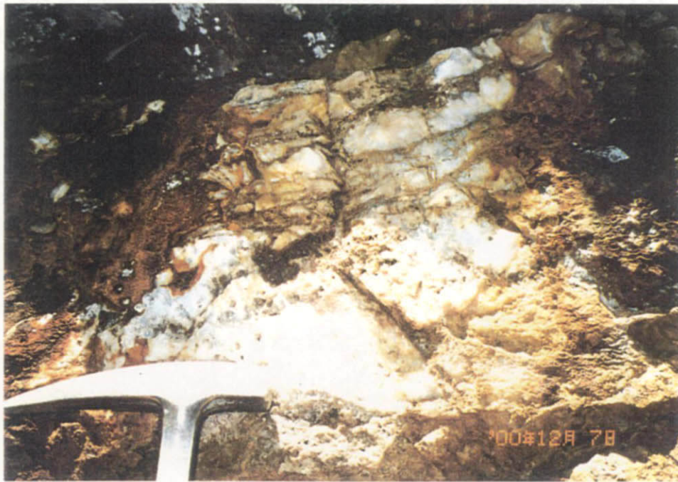
Plate 36 Epuyén district : Quartz vein with limonite in the mineralized outcrop of Plate 35. Chemical analysis revealed 9.14g/t Au.
