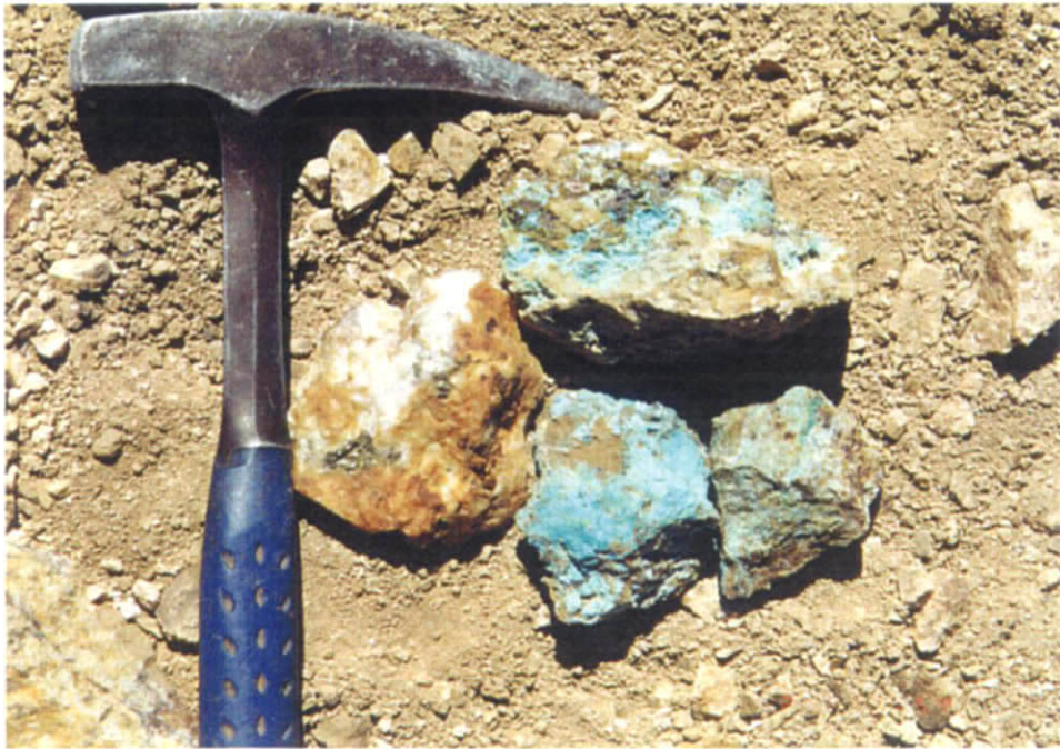
Plate 7 Varvarco district : Ore samples of chalcopyrite-bearing pyrite quartz vein (left) and quartz vein with malachite and azurite (right), collected in the stock pile of Mina Santos
