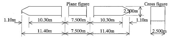
Fig. 6.1.1 Car Body Shape for the Calculation of Car Body Eccentricity
