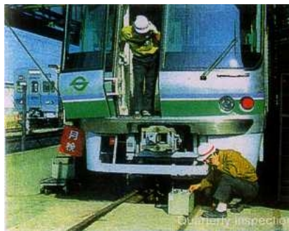
Fig. 5.1.46 Emergency Excite under Quarterly Inspection 06 series of subway rolling stock, Chiyoda Line, TRTA, Tokyo
