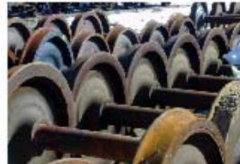
Worn Wheel Waiting for Cutting at Rajilovac Workshop
