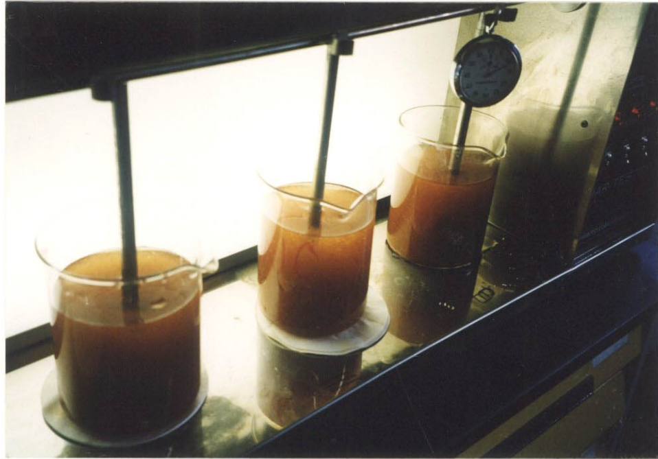
Photo. EIS-5 Jar Test (Coagulation/Sedimentation Test) at TIMS.
