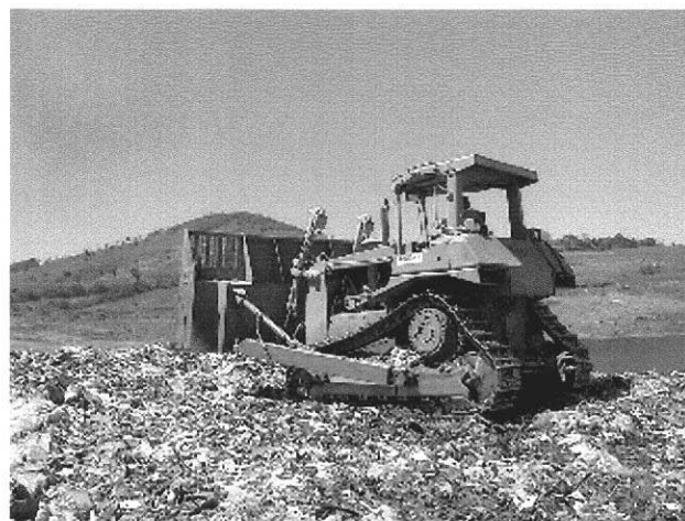
Waste are spread and compacted by a bulldozer in Nejapa Sanitary Landfill Site.
