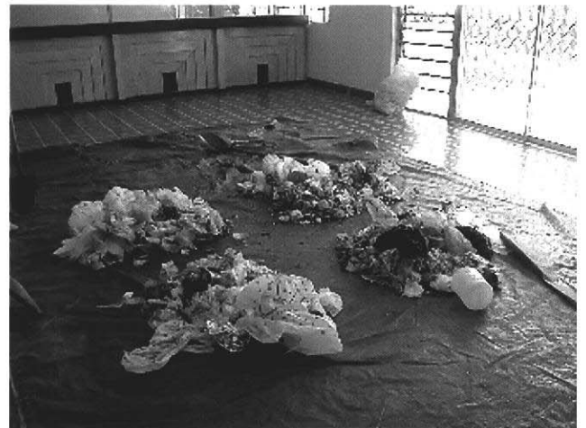
After proper mixing, the waste was divided into four segments of approximately the same size and this is repeated until the volume is reduced to the desired volume.
