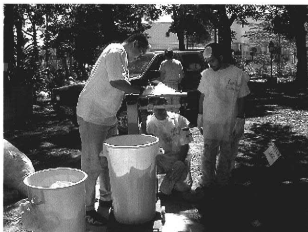
Waste samples were put into a calibrated plastic bucket to record volume and weight.
