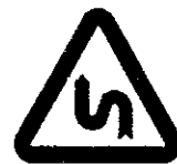
DOUBLE BEND ON SUCCESSION OF MORE THAN TWO BENDS THE FIRST TO THE LEFT W-4
