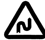
DOUBLE BEND ON SUCCESSION OF MORE THAN TWO BENDS THE FIRST TO THE RIGHT W-3
