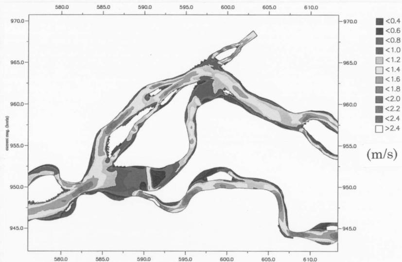
Contour of Current Magnitude (Alt. B2-3,  $Q=66,000 \text{ m}^3/\text{s}$ )
