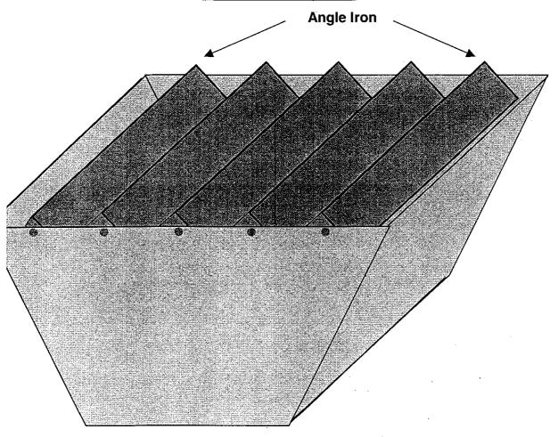
Orosses and fume "dumped" onto the skip open the swivel lids of "angle iron" to pass down into the skip. The angle iron lids swivel back into position and seal the skip.
