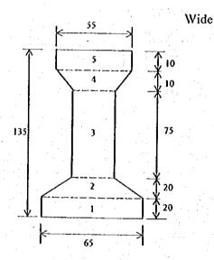
Length of Center Beam = 18.80 m Volume :  $A \times I$ ,  $V_1$ : 0.4575 × 18.80 = 8.601 m<sup>3</sup>
